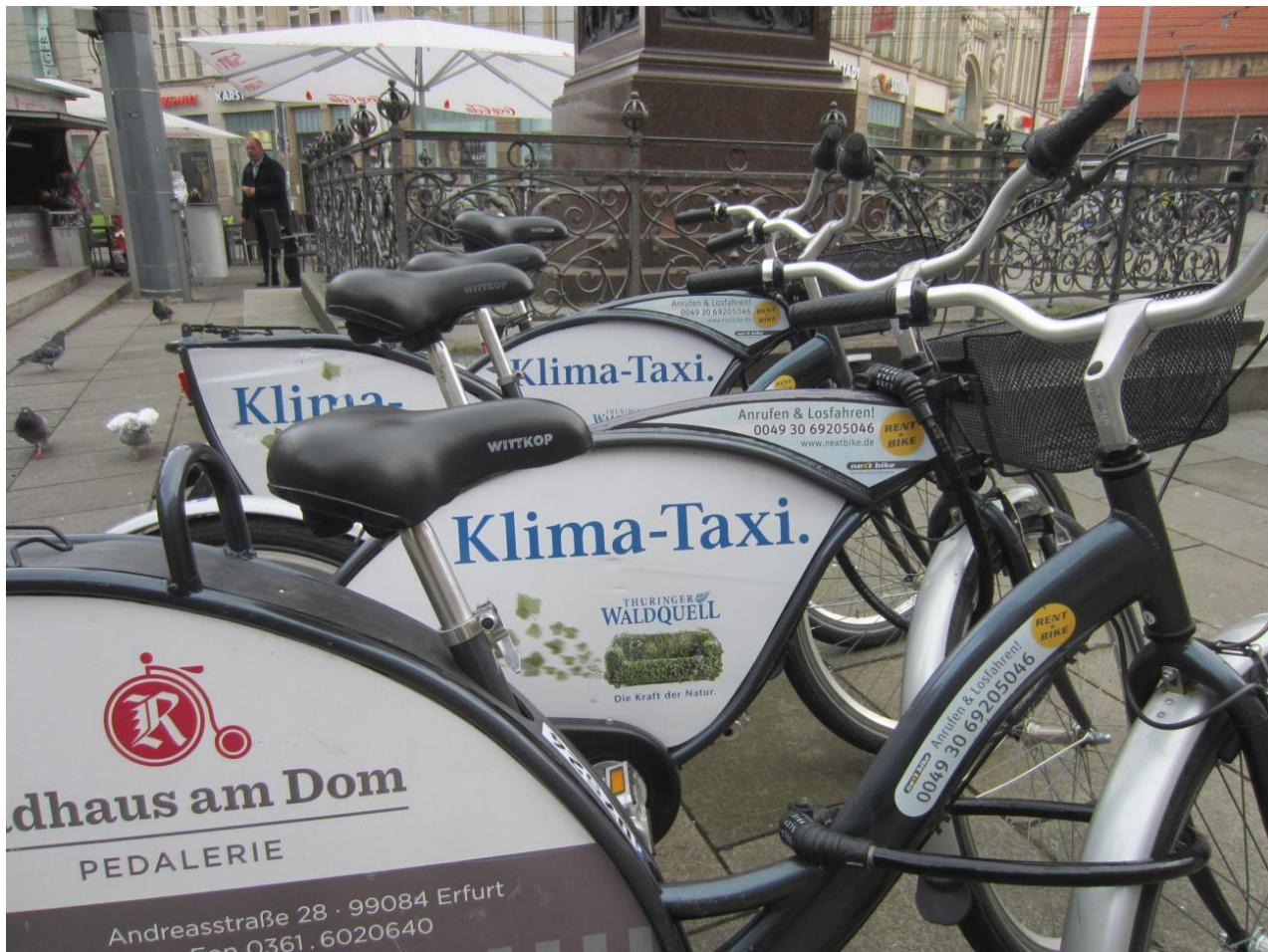
Figure. Klima-Taxi in Erfurt, Germany is a low cost measure that reduces the need for expensive docking bays and electronics. An SMS message gives the code for the bicycle and off you go. (Photo Jason Meggs)
